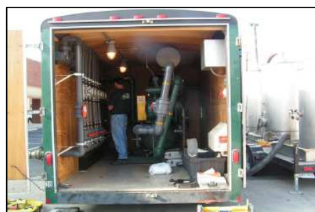
Figure 1. SVE Test. In October, EPA conducted an SVE test near suspected contamination sources. (Source: EPA)
