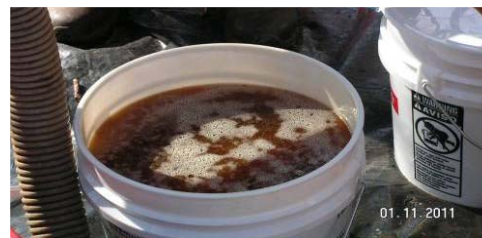
3DME applied to DW-404 in January 2011 as part of EPA's bioremediation study. (Source: EPA)
